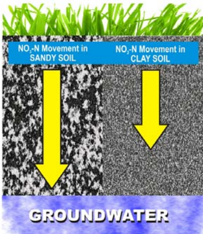
Nitrate is more likely to move downward in sandy soil than in clay soil.
